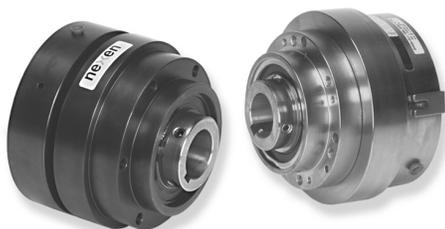
Nexen's **torque limiters** play an essential roll in safeguarding expensive web equipment and limiting down time by preventing damage during overload situations. The single piston, ball-detent design assures synchronized re-engagement in the same position every time. Operators can also manually position machinery by disconnecting the air supply to the torque limiter.
