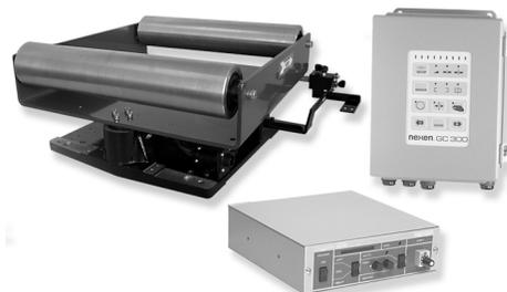
Nexen **web guiding systems** provide consistent lateral alignment to ensure quality operations. With a wide range of self-contained web guides for unwind, intermediate and windup processes, Nexen also offers **web guide controllers and amplifiers**. These units provide automatic positioning of the web by translating feedback from web sensors into control signals which are sent to the web control drive motors.
